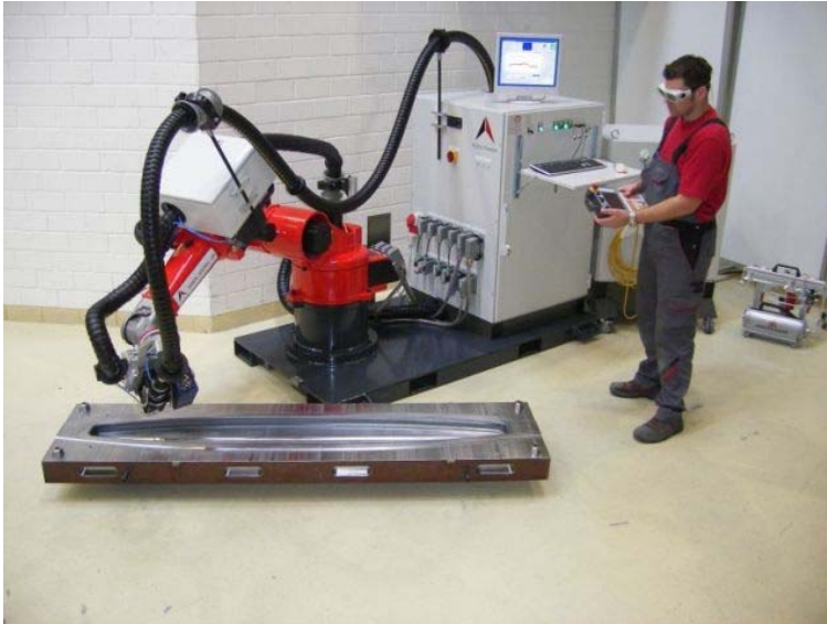
Figure 2 mobile laser hardening system at ALOtec Dresden
