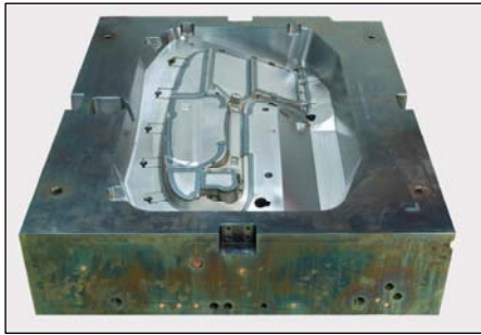
Figure 1 Partial hardening along the closing edge of a molding tool
